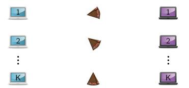
$$R_k^{\text{TDMA}} = \frac{1}{K} E_{\mathbf{H}} \left[ \log \left( 1 + \frac{K}{|h_{kk}|^2} P_k \right) \right]$$
