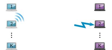
$$R_k^{\text{TDMA}} = \frac{1}{K} E_{\mathbf{H}} \left[ \log \left( 1 + K |h_{kk}|^2 P_k \right) \right]$$
