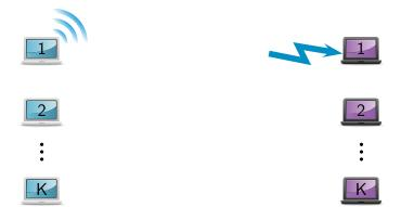
$$R_k^{\text{TDMA}} = \frac{1}{K} E_{\mathbf{H}} \left[ \log \left( 1 + \frac{K}{|h_{kk}|^2} P_k \right) \right]$$
