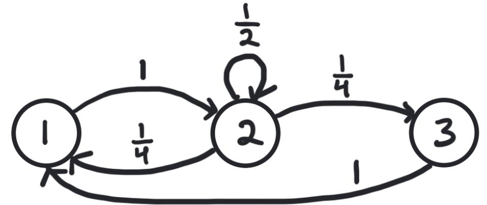
→ Calculate  $p_1 = P^T p_0 = \begin{bmatrix} 0 & 1 & 0 \\ 0 & 0 & 1 \\ 0 & \frac{1}{2} & \frac{1}{4} \end{bmatrix} \begin{bmatrix} \frac{1}{3} \\ \frac{2}{3} \\ 0 \end{bmatrix} = \begin{bmatrix} \frac{2}{3} \\ \frac{1}{3} \\ \frac{1}{6} \end{bmatrix}$
